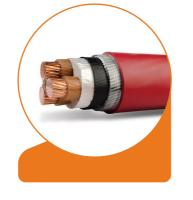
Description Soft stranded copper or aluminum conductors insulated with XLPE compound rated 90°C. Assembled together, armored with steel wire and sheathed with a PVC compound layer. Meets IEC 60502, BS 5467.
